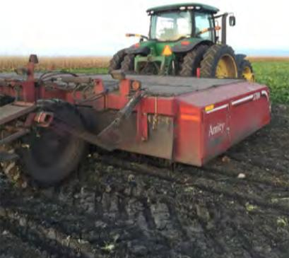
The rotobeeper travels in front of the harvester and removes the green tops.
